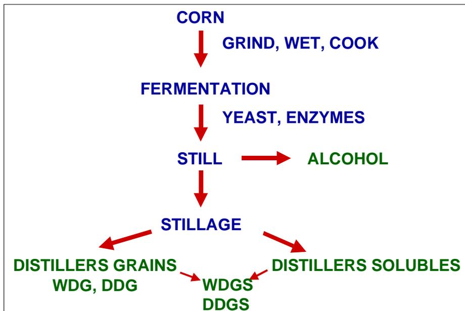
**Figure 2.** Schematic of the dry milling industry with the feed products produced.
