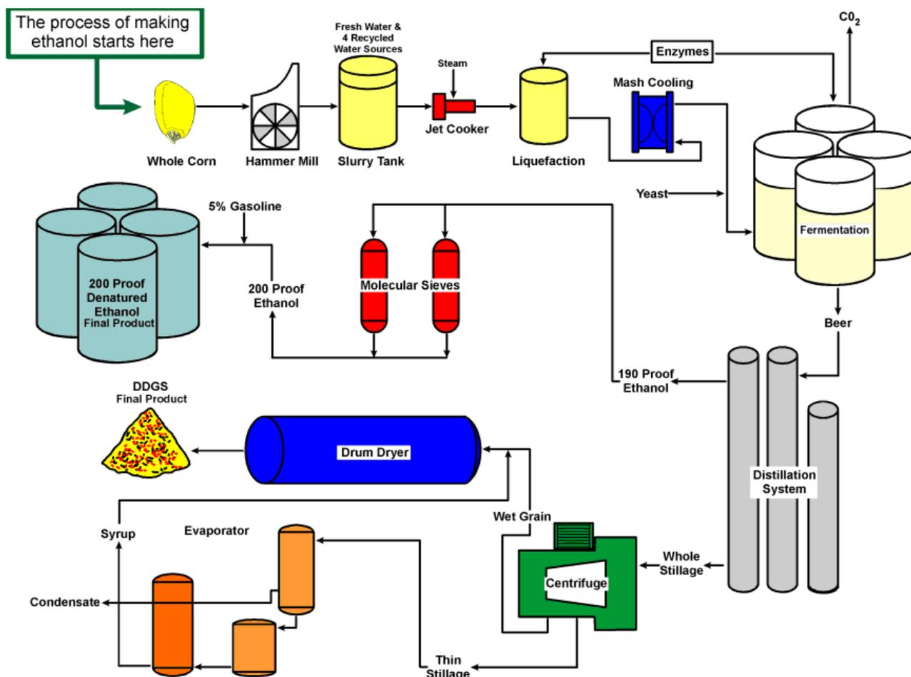
Figure 1. Dry-milling ethanol production process (www.exolmn.com/main.htm) [1]
