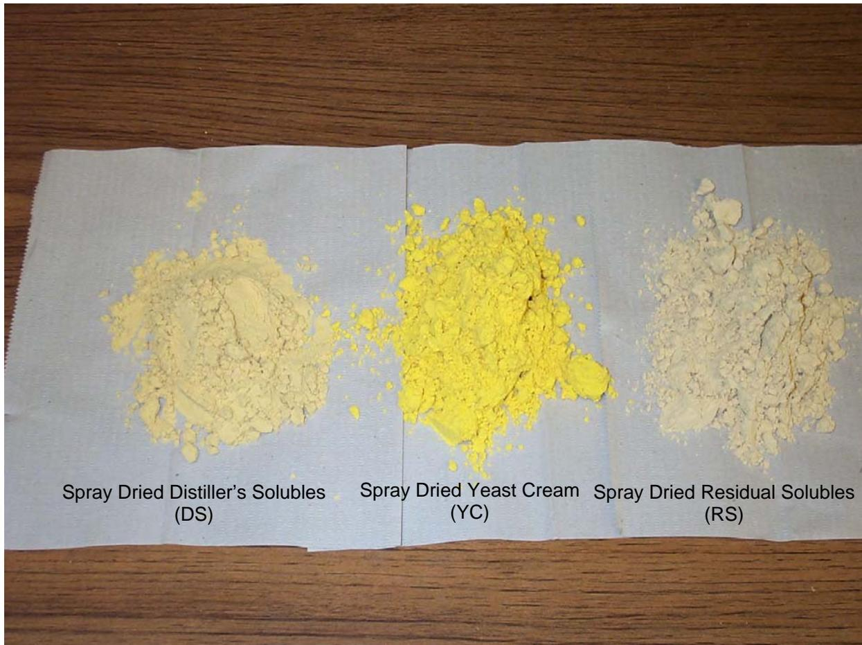
**Figure 10.** Appearance of spray dried distiller's solubles, spray dried yeast cream, and spray dried residual solubles.
