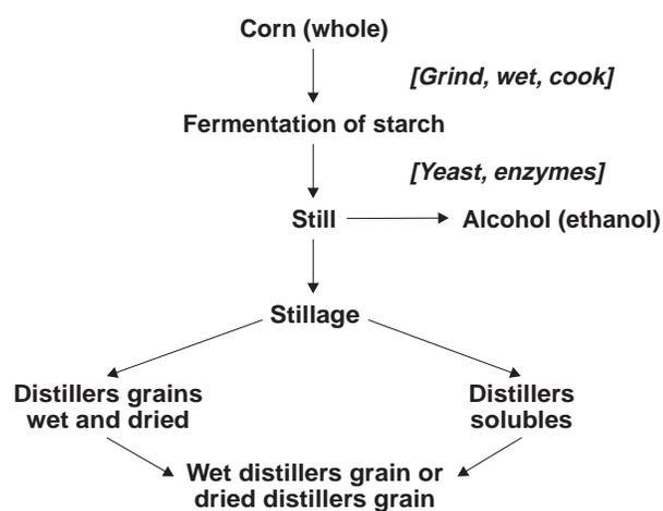
**Figure 1.** Schematic of the dry milling industry and the feed products produced.
