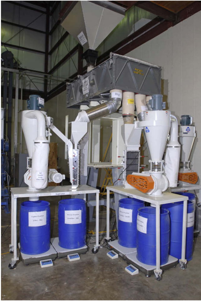
Fig. 2. Photograph of pilot plant for the Elusieve process.
