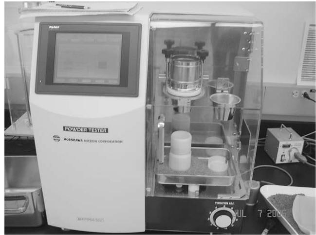
**Fig. 4 – Semi-automated tester for Carr indices.**
