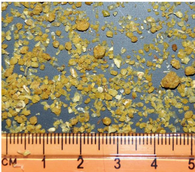
**Fig. 5.** Close-up photograph of a DDGS sample, showing different texture and shapes of particulate material.
