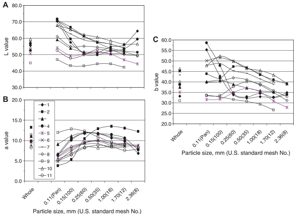
Fig. 4. Surface color, expressed in  $L$  (A),  $a$  (B), and  $b$  (C) color space, in the original (whole) and sieve sized fractions of the 11 DDGS samples.
