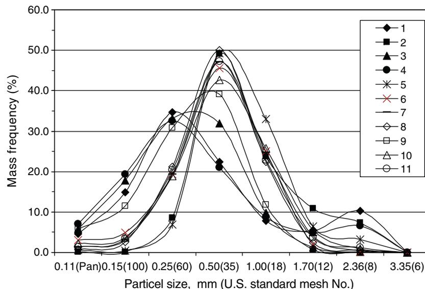
**Fig. 1.** Particle size distribution of 11 DDGS samples collected from the US Midwest region. Mass frequency was based on the proportion of material retained on each sieve size, by weight.
