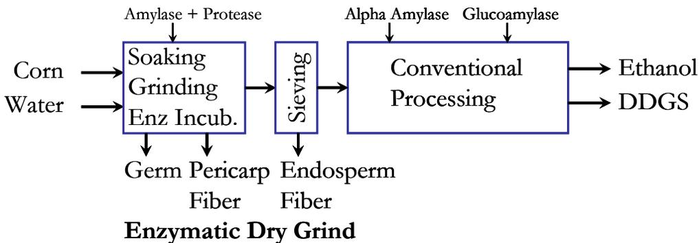
Figure 6. Modified dry grind corn processes (Singh et al 2005).
