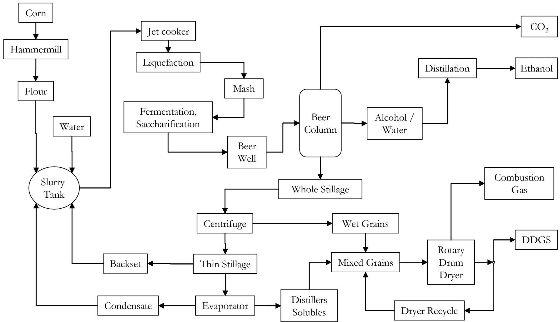
Figure 4. The dry grind corn process.
