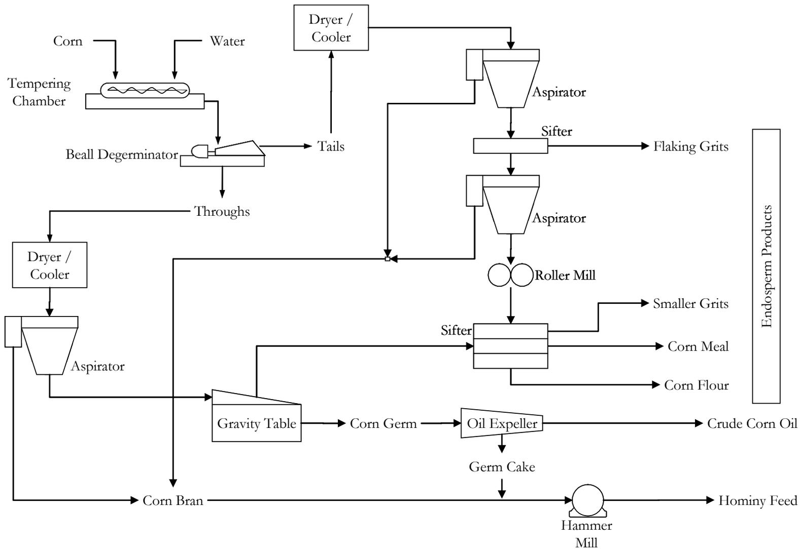
Figure 5. The corn dry milling process.
