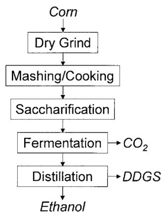
Figure 1—Dry-grind ethanol production process.
