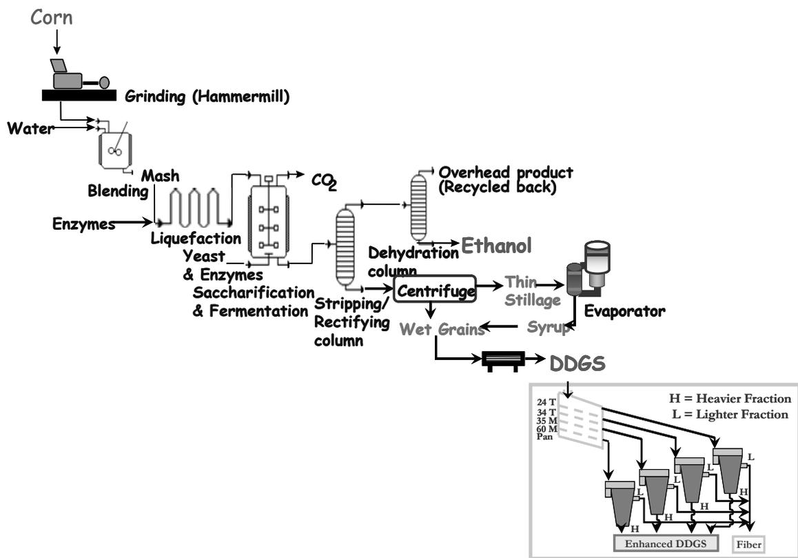
**Figure 4. Elusive process to remove fiber from DDGS.**
