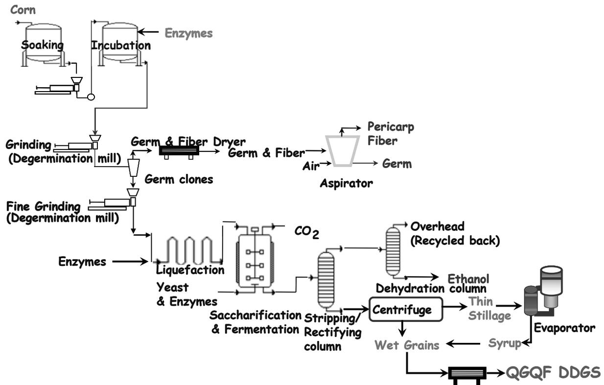
**Figure 2. Enzymatic (E-Mill) dry grind corn process.**
