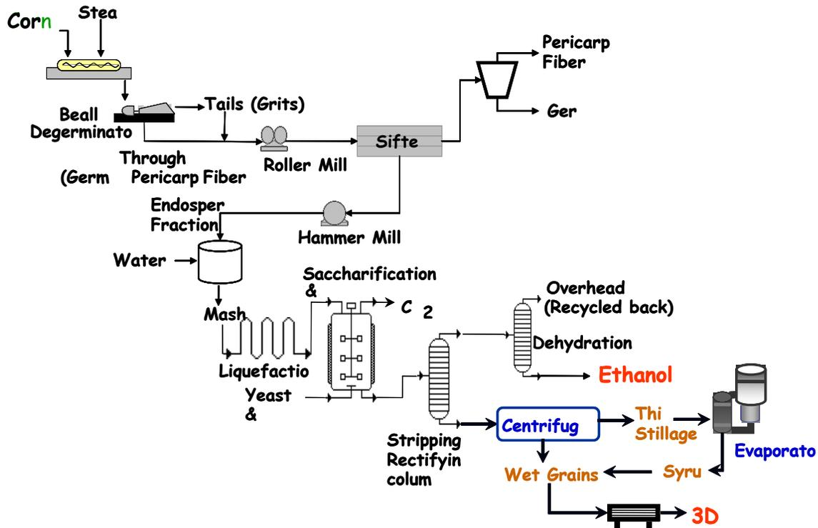
**Figure 3. The dry degerm defiber (3D) process.**
