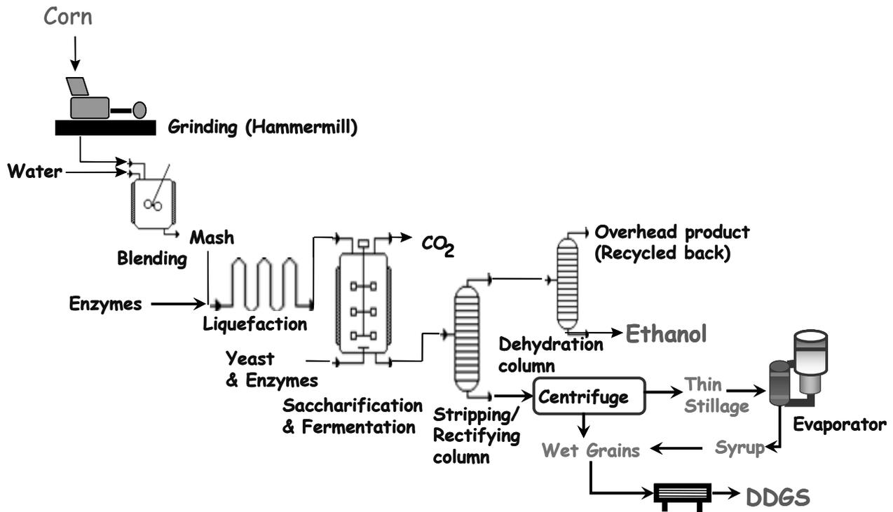
**Figure 1. Conventional corn dry grind process.**
