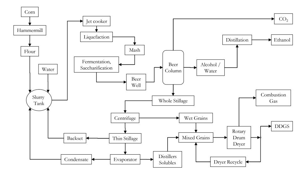
Figure 4. The dry grind corn process.
