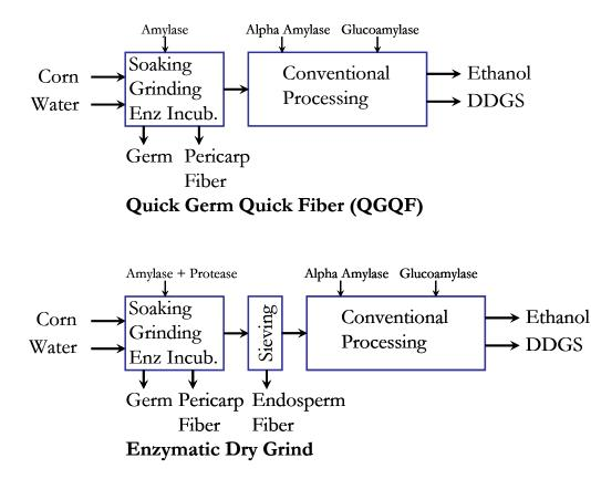
Figure 6. Modified dry grind corn processes (Singh et al 2005).
