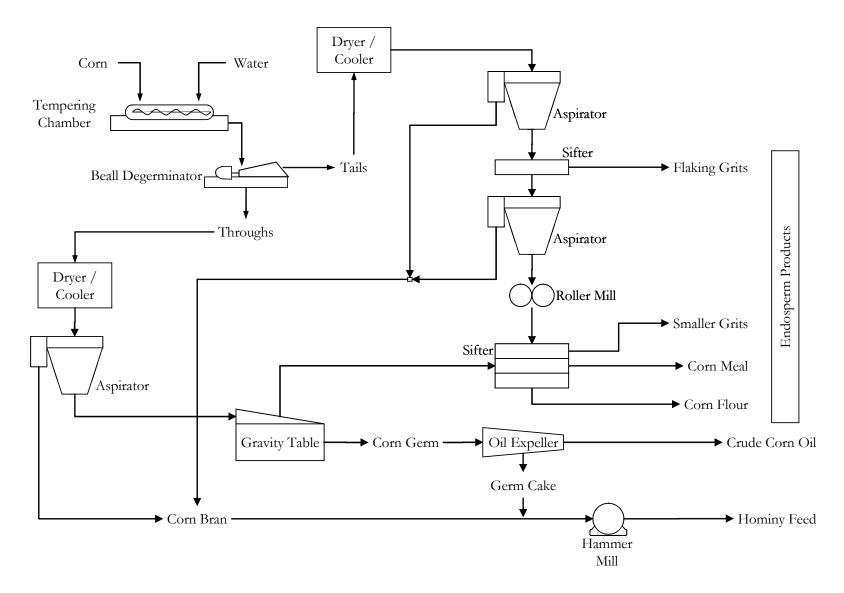
Figure 5. The corn dry milling process.
