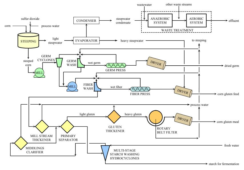
Figure 3. The corn wet milling process.
