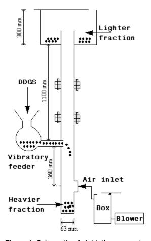
Figure 1. Schematic of elutriation apparatus.
