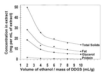
Figure 3–Effect of ethanol volume on the concentration of total solids, fat, glycerol, and protein in the extract.
