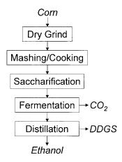
Figure 1–Dry-grind ethanol production process.
