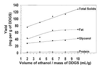
Figure 2–Effect of ethanol volume on the yield of total solids, fat, glycerol, and protein from DDGS.
